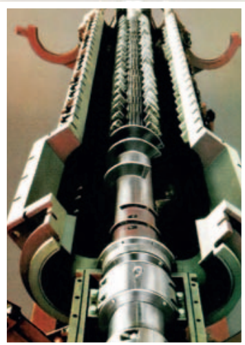
Complete continuous mixer/kneader with oscillating gearbox.
